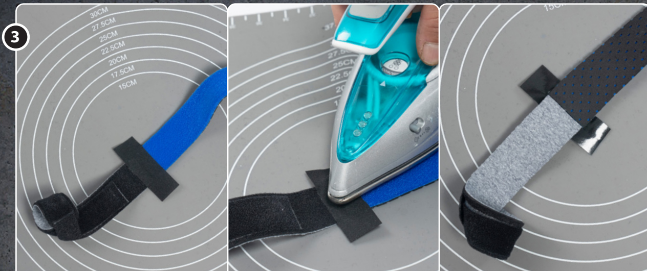
3 Cut a 6-7 cm long 22 mm NRX® Heat Tape and cover the joint. Before affixing it, check that the joint does not have a gap. Apply the tip of the iron over the joint, holding for about 5 seconds. Let the tape cool to stabilize for 30 seconds and then turn the construction.
