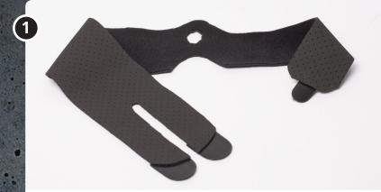
Cut a 35-40 cm length of the NRX® 110 mm strap. In the middle of the strap, cut a hole for the thumb, off center. Under the thumb hole you cut a curve. The space between the top of the curve and hole should be 15-25 mm. Cut a shaped curve from the 10-15 mm from the top of the hole and angle it towards the end of the strap on one side. Do the same on the other side but keep this part slightly wider. Splint the end of that part.
